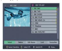
Use the [LEFT] or [RIGHT] keys to highlight the FAVOURITE button at the base of the screen and then, in turn, highlight each channel that is required to be a favourite channel, using the [UP] and [DOWN] keys (and the [PAGE UP] or [PAGE DOWN] keys), and press [OK]. A channel selected as a favourite appears in the main channel list with a favourites icon against the channel name.
