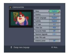
The various configuration functions are displayed in a list, along with a quarter-screen image of the currently selected channel. You can select a function by highlighting the corresponding menu line with the [UP] or [DOWN] keys. There are seven configuration functions.
