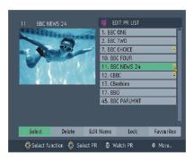
Here, you can preview any channel stored by the receiver before viewing it full screen. The complete list of channels is displayed in pages of 11 channels at a time, with their channel list number and a favourite channel icon if appropriate (see -ADVANCED OPERATION - Favourite Channels). The name and a quarter-screen image of the channel last viewed is displayed in the top right of the screen.
