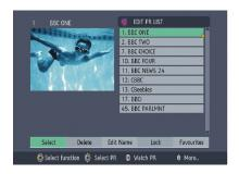
The Channel List screen displays the list of channels in the receiver's memory, with a quarter-screen image window showing the selected channel, and can be used to change channels for viewing, delete channels from the memory, edit the name of the channel as it appears in the list and on-screen, lock a channel against viewing by younger members of the family, and set up favourite channels.
